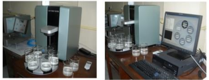
Gambar 1. Fiber analyzer Lorentzen wette
